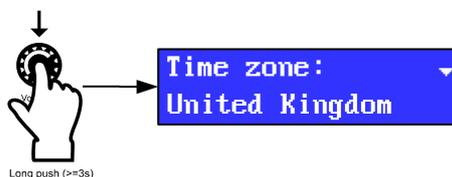
The first line displays the name of the time zone setup sub-menu. The second line displays the active time zone rule: either a geographical rule (i.e. a country, with a region if any), or a constant UTC-relative offset.
