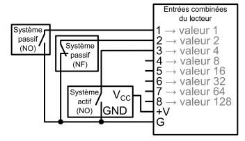
their combination, defined as the sum of the values of all the active inputs, which is simply the value of an input if it is the only one active. If more than 8 triggering devices are needed, the Waves System Ext15In board or a diodebased circuit can be used to get more than 8 combinations from these devices.
